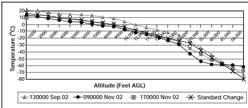
Figure 5: Temperature vs Altitude for Three Different Days
